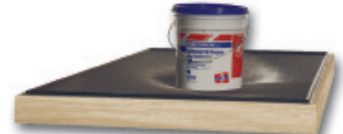
67 pound bucket placed on the screen panel for 21 days...then removed
